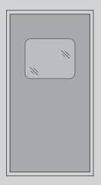
Sheet panel with 1.2 mm thickness with portlight gasket. It can be produced with frame 20x20 or 30x30.
