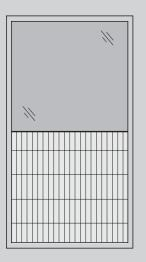
22x100 mesh panel and extremely tough transparent material with thickness 4 mm. It can be produced with frame 20x20 or 30x30
